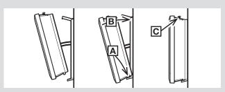
NOTE: If you need to remove the thermostat, follow step 1 in section 1, then use a straight screwdriver to unhook it from the top of the mounting plate.
